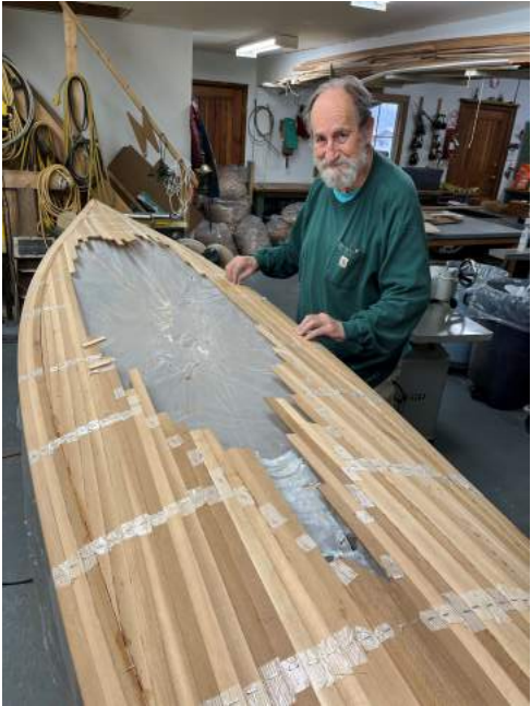
Charlie securing the last strip on his stitch and glue kayak
